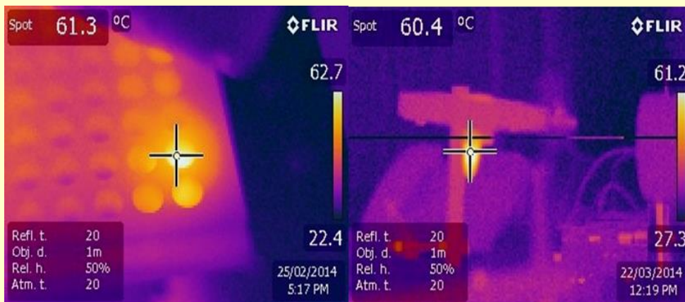
Infra red (IR) thermal images of GNR samples in microplate wells (Left Panel) or centrifuge tube (Right Panel) exposed to the NIR laser at power density of 1.05 W/cm 2 . Within the panel cursor represents spot temperature and the vertical pseudo-color bar signifies temperature intensity from high (yellow) to low (dark blue).
